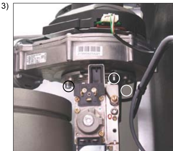
3) Undo the mixing chamber from the fan (three Allen screws 5 mm), and remove air inlet pipe where necessary
