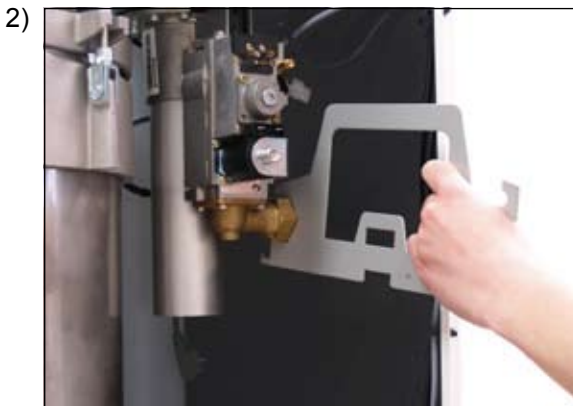
Undo gas connection at the gas combination valve
